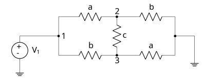
Start by finding the equivalent resistance. The easiest way to do this is to replace the voltage source with a current source I, and then find the voltage  $V_1$  at node 1. The equivalent resistance is then  $V_1/I$ . This involves solving 3 equations for nodes 1, 2 and 3. The equations are Kirchoff's current law applied to the nodes. Leaving out the details, the equivalent resistance is
