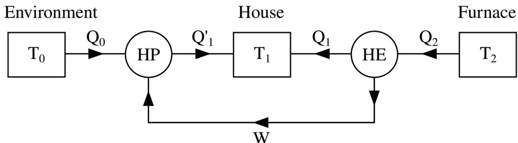
There are three heat reservoirs, the outside environment at temperature  $T_0$ , the inside of the house at temperature  $T_1$ , and a high temperature heat source at  $T_2$ . The high temperature source could come from the combustion of some fuel such as natural gas. There is a heat engine operating between  $T_2 \gg T_1$  that produces work  $W$ . This work is used to drive the heat pump that operates between  $T_1 > T_0$  pumping heat into the house.
